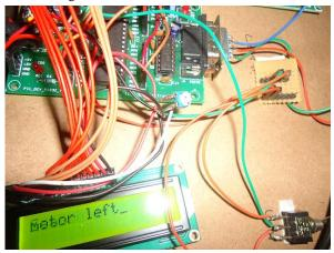
Fig: 13. Rotation of Left Motor
