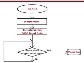
Fig: 10. Activation of Pic controller
