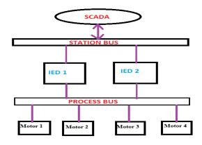
Fig: 1. The SCADA Connected to IEDs Through Buses
